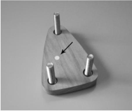
Now place your free hand on the three round nuts to prevent them from slipping and turn with your hand the wooden panel. The side with the colored sticker is facing you now. Place the wooden panel like that in front of you. The panel lies now on the round nuts. The threaded rods face upwards.
