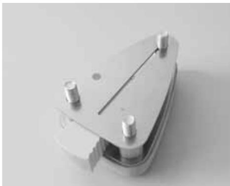
Take the second stainless steel inlay in your hand. Grasp the stainless steel inlay so, that with the label marked side facing upward. Run the stainless steel inlay on the threaded rods and place it on the stainless steel bushings. Please ensure that the steel pin in wooden wedge also performed in the second slot of the stainless steel inlay.
