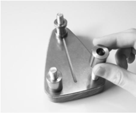
On the threaded rod into the top of the triangular wooden panel insert the stainless steel socket with a groove. On the two threaded rods at the short side of the triangular wood cheek insert now the stainless steel sockets (without groove).
