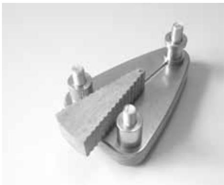
Place now the wooden wedge, which is inserted already with the imported steel pin with smooth sides on the already mounted stainless steel inlay. Place the wooden wedge so, that the protruding steel pin in the slot of the stainless steel inlay must be performed.
