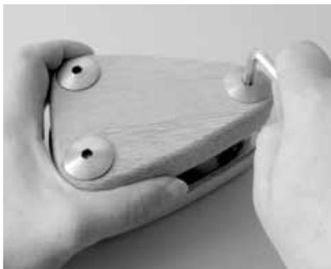
Now screw the three remaining round nuts with the three threaded rods, which are placed in the holes of the second wooden panel. As tool you can also use the Allen key from the delivery. Finally drag every six round nuts tightly. In front of you is now the fully assembled height adjustment for your TRAUMSCHWINGER.
