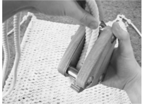
Now take the height adjustment so in your right hand, the wood wedge almost half inserted into the height adjustment. Insert the end of the rope pair as the left stainless steel bushing of height adjustment, that two ropes side by side laying on the stainless steel bushing.
