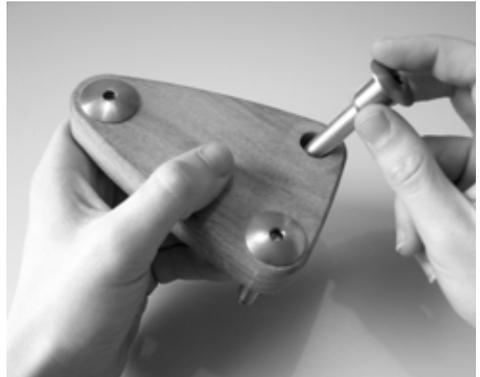
Take now one of the triangular wooden panel. One side of the wooden panel is marked with a colored sticker. That is the inside of the panel. Hold the panel with one hand, so that the sticker marked side faces downward. With your other hand put through each of the three holes a threaded rod with a round nut.
