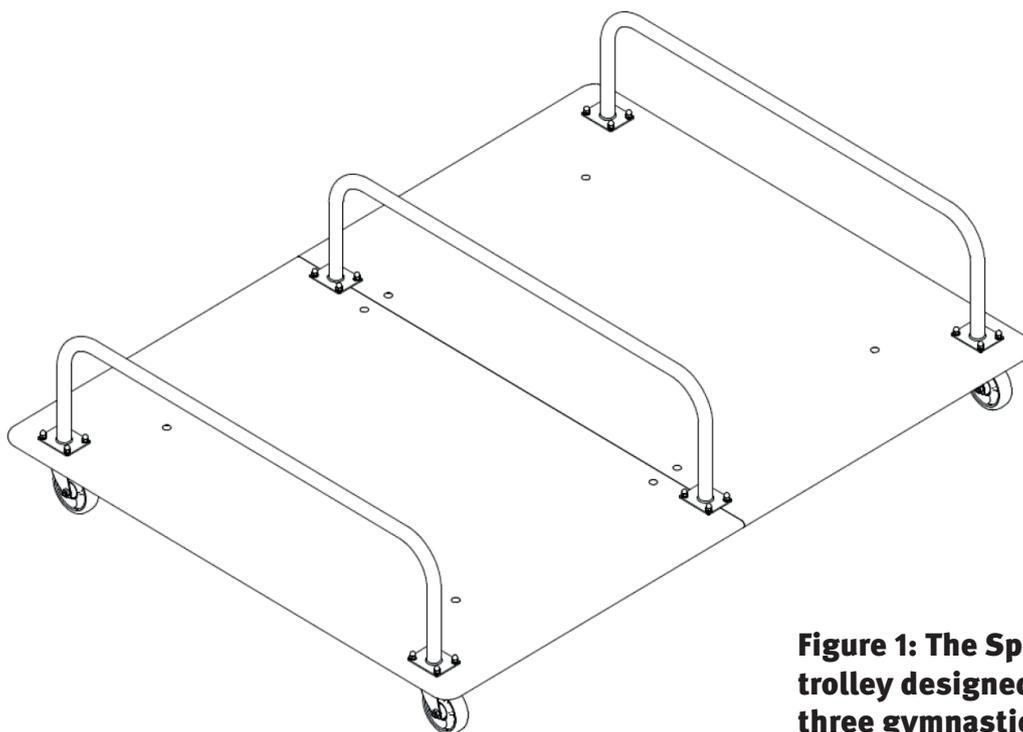
**Figure 1: The Sport-Thieme trolley designed to hold three gymnastics mats.**
