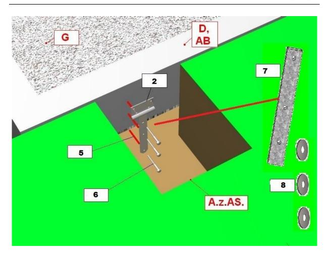
Please pre-drill the appropriate position with the stone drill (pos. 10). After that please install the dowel, the tilting hinge and screw on the pipe reinforcement with Pos. 6.
