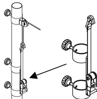
III. 4: Safety tensioning device \*
