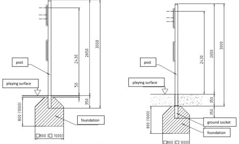
Illustration 2: Foundation (without and with ground socket)
