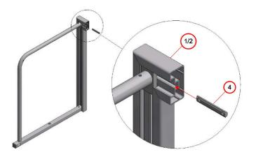
1. Slide a slot nut double M8 (3) in the little groove of the goal post elements, that a half of the slut nut look out.
