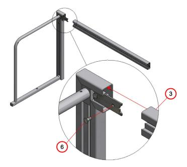
3. The crossbar (3) slide on the lookout connector (5) and slot nut. The countersunk screw M8x16 (6) tighten loosely through the connectors.
