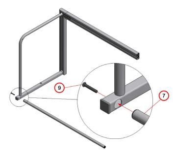
4. Put the ground frame tube (7) in the openings of the goal post element (1)
