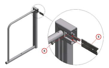
2. Slide two connector (5) in the big groove and align the bore holes of the connector (5) to the slot nut (4). The countersunk screw M8x20 (6) tighten through the connector into the slut nut.
