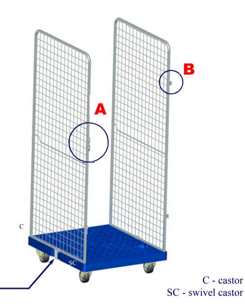
Mount back panel and fix to the side mesh panels (left & right) using the plastic clips.
