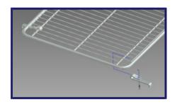
Push support bracket over wire Ø 8 mm and fix with bolt M6 x 25 mm and nut M6.
