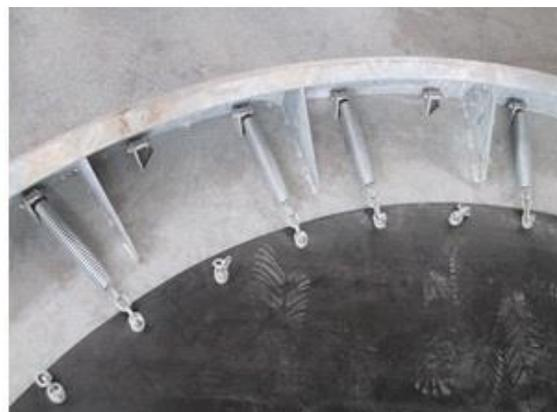
**Place the first tension spring in the membrane opposite the tensioning strap.**
