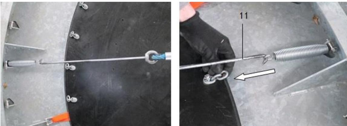
**Chain links must not be twisted when the tension spring is inserted**
