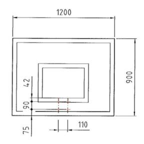
On the drilling diagrams to the right, you can see the positions of the holes that still require drilling. For basketball backboards with the dimensions:
