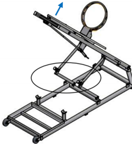
Figure 4: Erecting the frame
